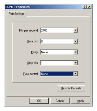
Choose 2400 baud, 8 bits, no parity, 1 stop bit and no flow control, then OK
